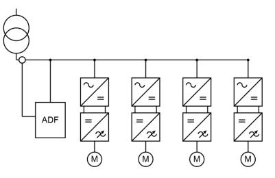
As indicated in the diagram above, the global compensation option is completely decoupled from the load, which increases flexibility during planning and installation. It also means the drives and filters can be installed, serviced and maintained independently of each other.
